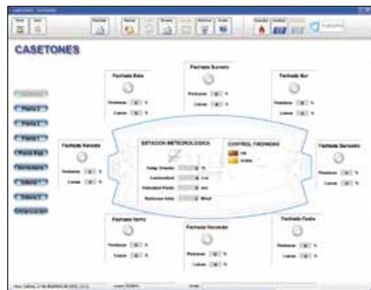
Visualisation example: The menu page of the weather station provides information about the external temperature, brightness, wind speed and solar radiation as well as the status of the eight façade sections.
