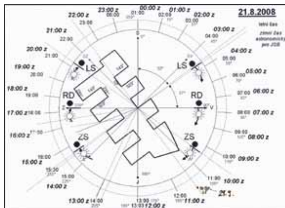
Sun protection precisely according to the daily routine: schematic from astro control
